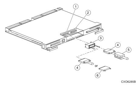
Figure 2–1. Cabling for a Single-Controller Configuration
